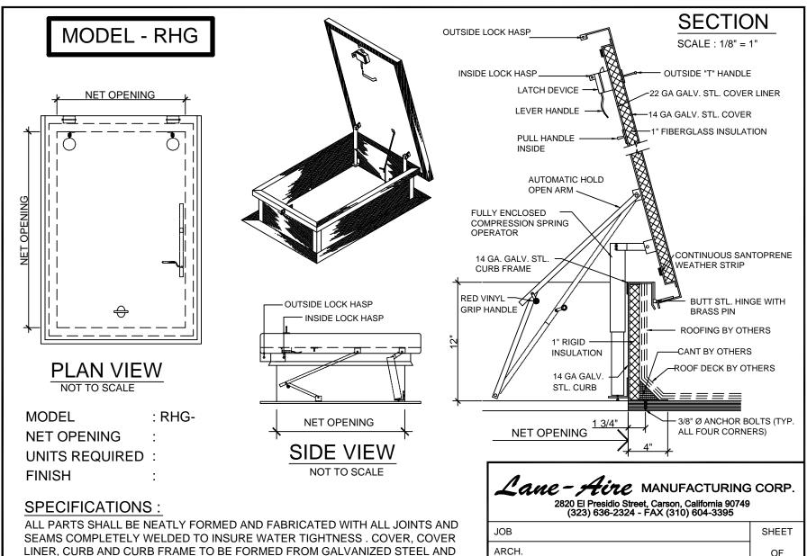
ALL PARTS SHALL BE NEATLY FORMED AND FABRICATED WITH ALL JOINTS AND SEAMS COMPLETELY WELDED TO INSURE WATER TIGHTNESS. COVER, COVER LINER, CURB AND CURB FRAME TO BE FORMED FROM GALVANIZED STEEL AND SUPPLIED WITH A GREY METAL PRIMER FINISH. UNIT SHALL BE SUPPLIED COMPLETELY ASSEMBLED AND READY FOR INSTALLATION. UNIT WILL OPEN TO MAXIMUM 75° POSITION. ACTUAL NUMBER OF SPRING OPERATORS TO BE DETERMINED AS NEEDED FOR SMOOTH OPERATION OF UNIT.
